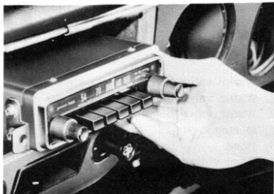
Fig. 4-3 Removing Radio Tuner B 2360
